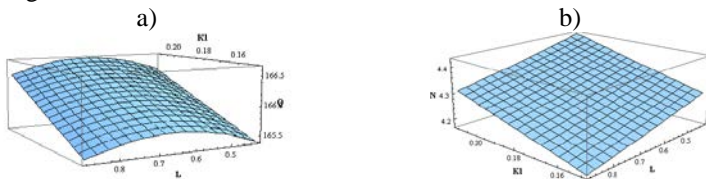
Figure 2. The effect of value of loading grinding bodies first chamber at Q, N, q , at different length, ( \varphi_2 = 0.3 ; \xi = 0 ; \alpha = -30^\circ )
